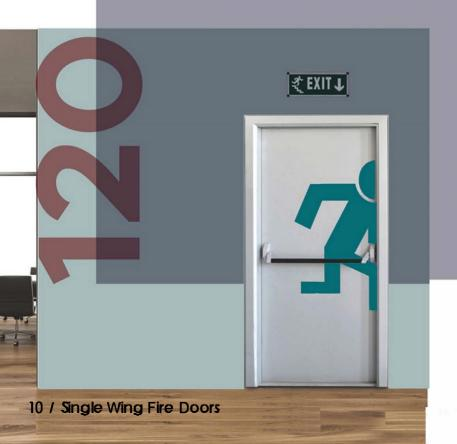
Standard EN 1634-1 Fire Resistance E Class: 120 Min. El Class: 120 Min. Width: Max. 1150 mm **Dimension** Height: Max: 2250 mm 1.5 mm DKP or Galvanised Fra me 1 mm DKP or Galvanised Wing Wing Thickness 66 mm 150 kg/m3 Rockwool, Isolation 128 kg/m3 Seramic Wool Kerafix Intumesan Seal Fire Seal 3 pcs hinges, one of Self-Spring, all of Twisted from 3 mm Mentese Sheet Metal
